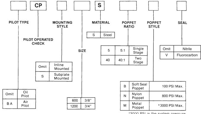
\*3000 PSI is the system pressure rating. The pilot pressure rating is 80 PSI for Air Pilot, 1000 PSI for Oil Pilot 1200 size and 3000 PSI for Oil Pilot 600 size.
